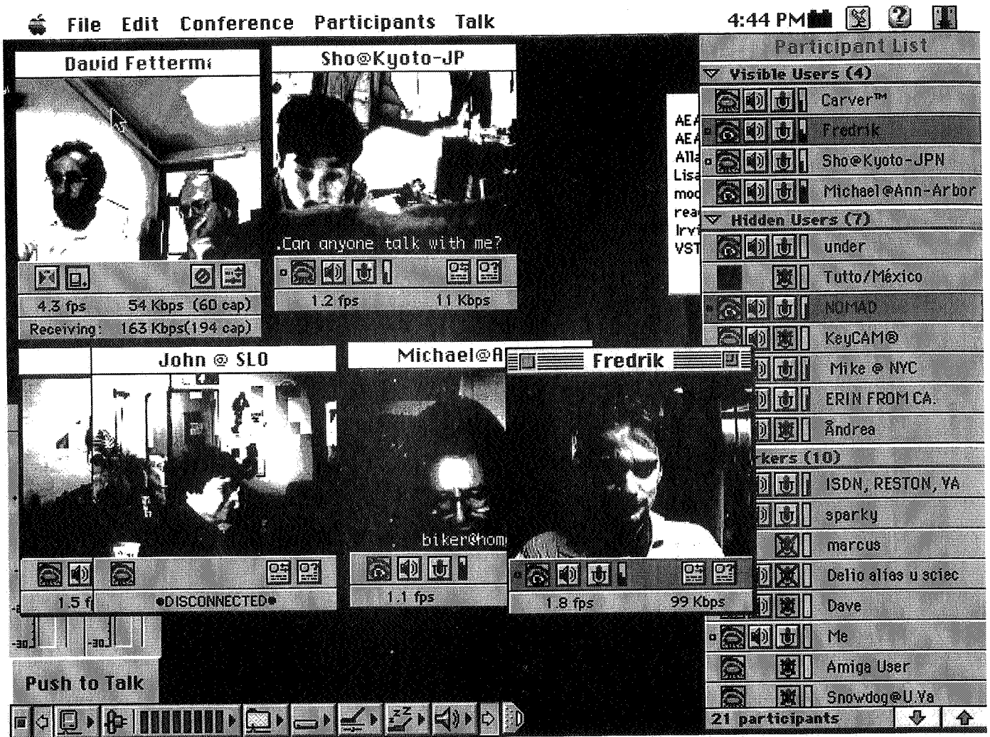
FIGURE 1. Computer screen snapshot of colleagues speaking to one another from Stockholm, Seoul, New York, San Diego, Tokyo, and Stanford. Colleagues can see one another by selecting a participant from the "participant list" in the right-hand column—initially under "hidden users." Once selected, "hidden users" become "visible users." Colleagues can speak to the entire group by pressing the "push to talk" button in the bottom left-hand corner. Selecting the microphone icon under each picture allows individuals to speak to one another privately.
